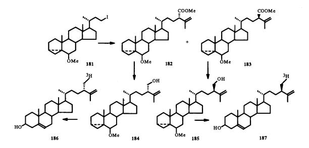
$[26^{-14}C]$ Codisterol (193) and  $[26^{-14}C]$ epicodisterol (194) have been synthesized from the 23-iodide (181) [45]. When this iodide was condensed with ethyl 2-methylacetylacetate, the ketoester (188) was obtained in a yield of 71%. Hydrolysis of the ester function followed by decarboxylation, taking place on the interaction of compound (188) with potassium hydroxide in ethanol, led with an overall yield of 88% to a mixture (1:1) of the 25-keto derivatives (189) and (190).
