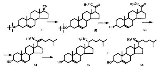
The  $\Delta^{20(22)}$ -derivative (54) has been synthesized by the Wittig condensation of the 20-ketone (53) with the corresponding phosphorus ylide in dioxane. Hydrogenation of the more accessible 20(22)-double bond in compound (54) over a platinum catalyst in a mixture of dioxane and acetic acid formed [21-<sup>13</sup>C]cholesterol (55) and its (20S)- isomer (56), which were isolated from the reaction mixture by high-performance liquid chromatography with yields of 43 and 13%, respectively.
