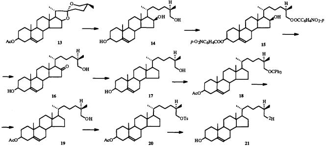
protective grouping in compound (18) with hydrochloric acid in ethanol led to the 26-alcohol (19), the tosylation of which with p-toluenesulfonyl chloride in pyridine gave the 26-tosylate (20), and this was reduced with lithium tetradeuterioaluminate in ether to the required (25S)-[26-<sup>2</sup>H]cholesterol (21).
